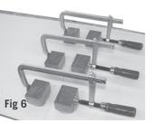
8. Adhesive excess must be removed at this stage from the joint before it hardens. Take care when doing so to ensure the join remains fully closed. Adhesive overspill elsewhere on the surface may be wiped off using denatured alcohol. Go across the joint with a ruler or similar to feel if a step exists, if a step is found then tap down until both sides are flat and level and re-tighten clamps. Ensure that you clean with denatured alcohol.
